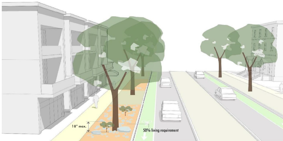
Figure 24-8-3: Streetscape — Pedestrian frontages.
