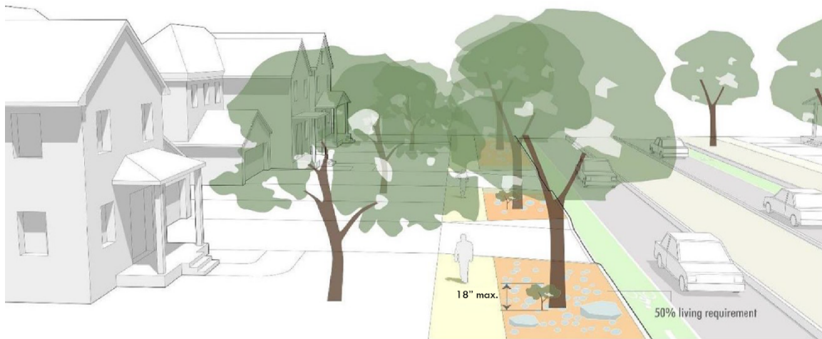
Figure 24-8-5: Streetscape — Residential frontages.
