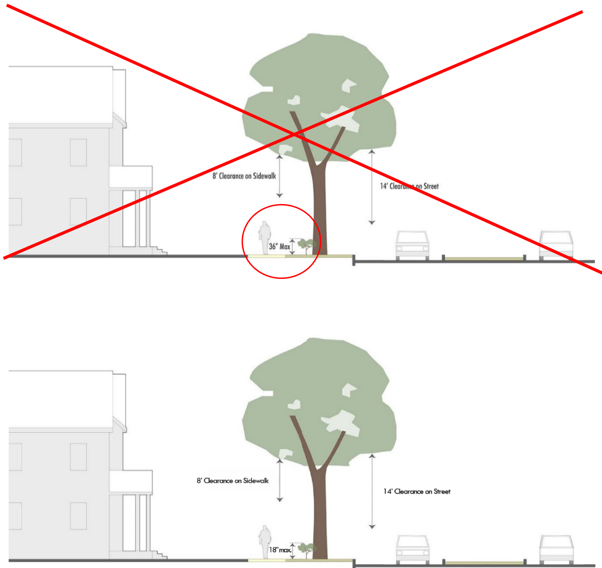
Figure 24-8-6: Tree clearance — Residential frontage.
