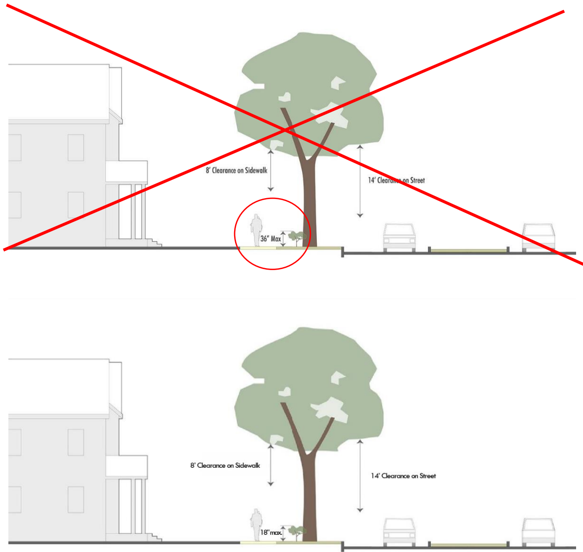
Figure 24-8-6: Tree clearance — Residential frontage.
