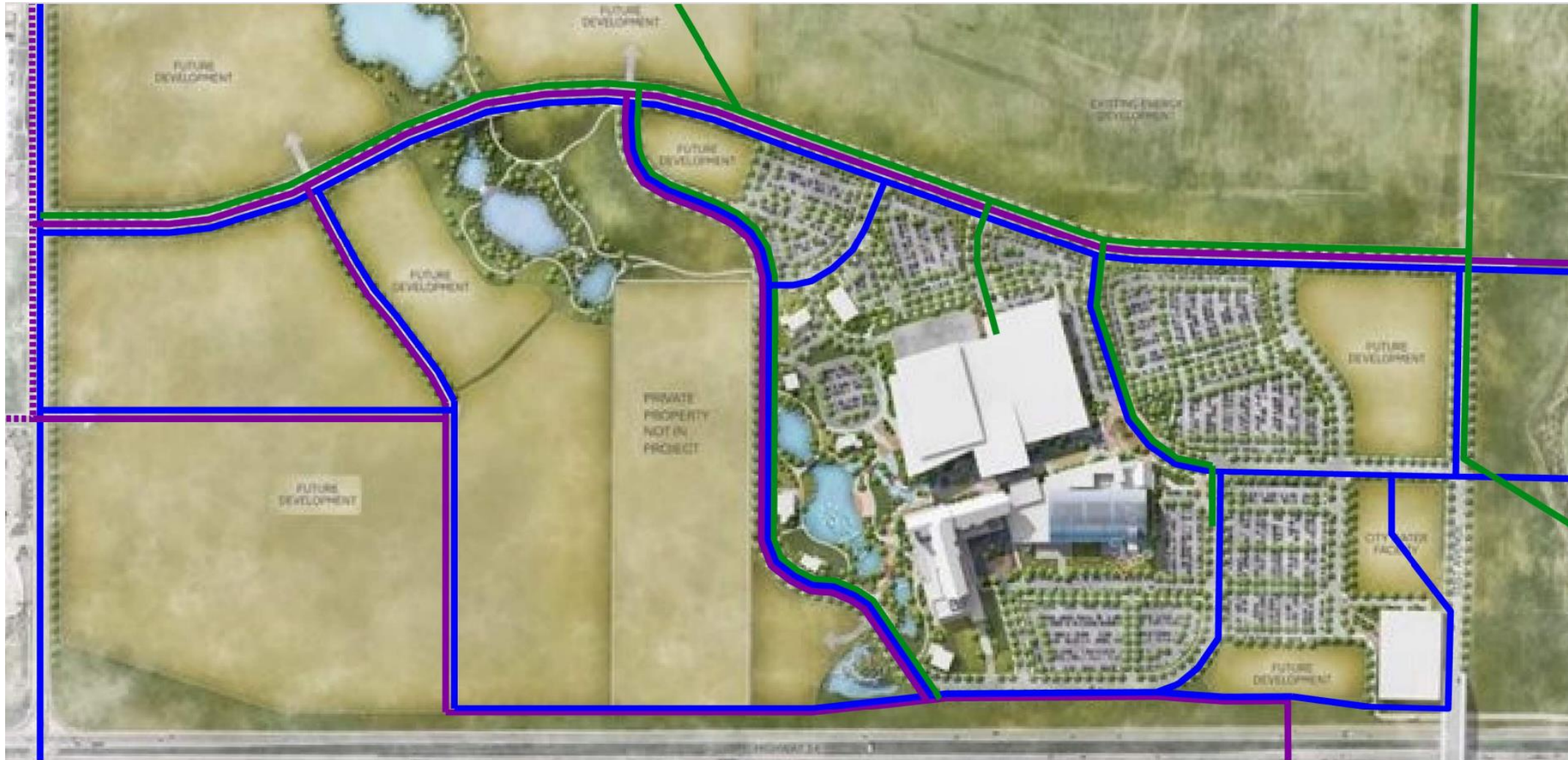
Concept plan map with core water & sewer infrastructure overlay
