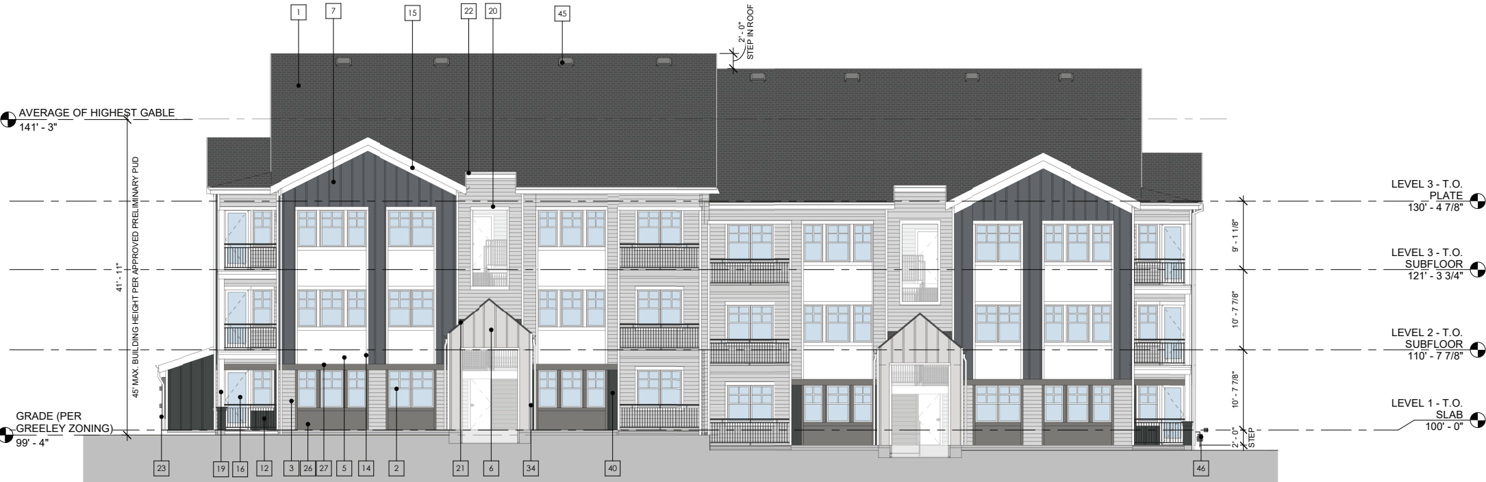
1 BUILDING D - FRONT ELEVATION 1/8" = 1'-0" SITE PLAN BUILDING: 6
