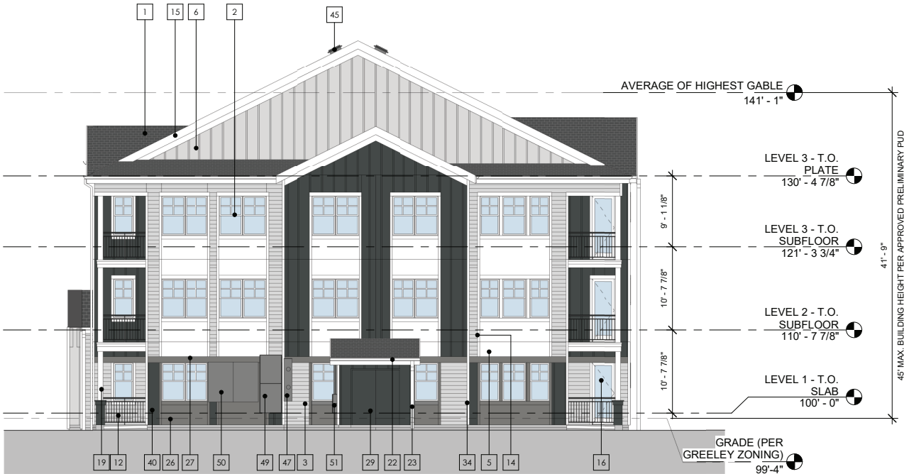
2 BUILDING B - RIGHT ELEVATION 1/8" = 1'-0" SITE PLAN BUILDING: 4,7,8,9
