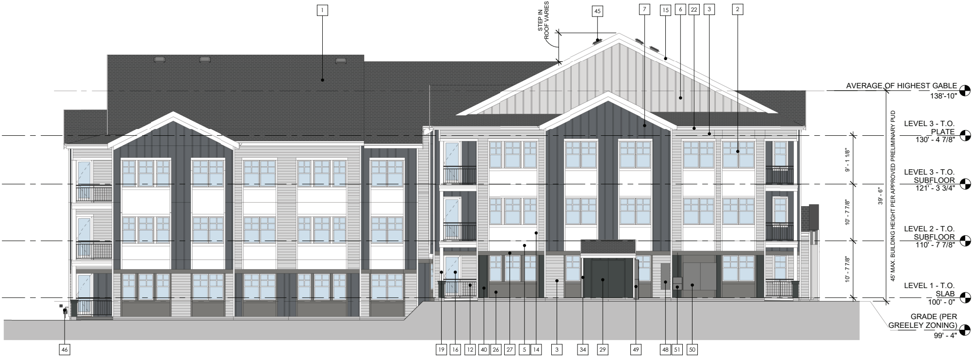
1 BUILDING A - LEFT ELEVATION 1/8" = 1'-0"
