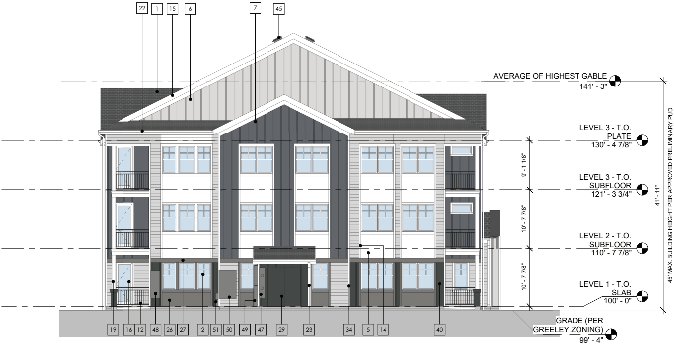
2 BUILDING D - LEFT ELEVATION 1/8" = 1'-0" SITE PLAN BUILDING: 6
