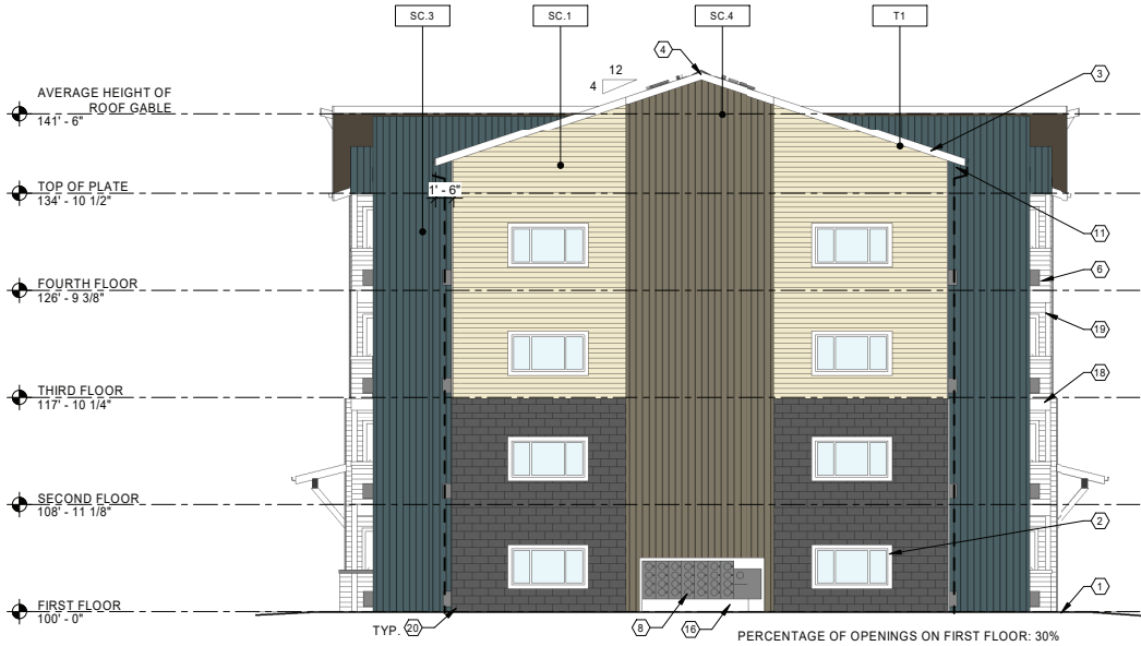
1 BUILDING TYPE 3 - END ELEVATION (NORTH)
