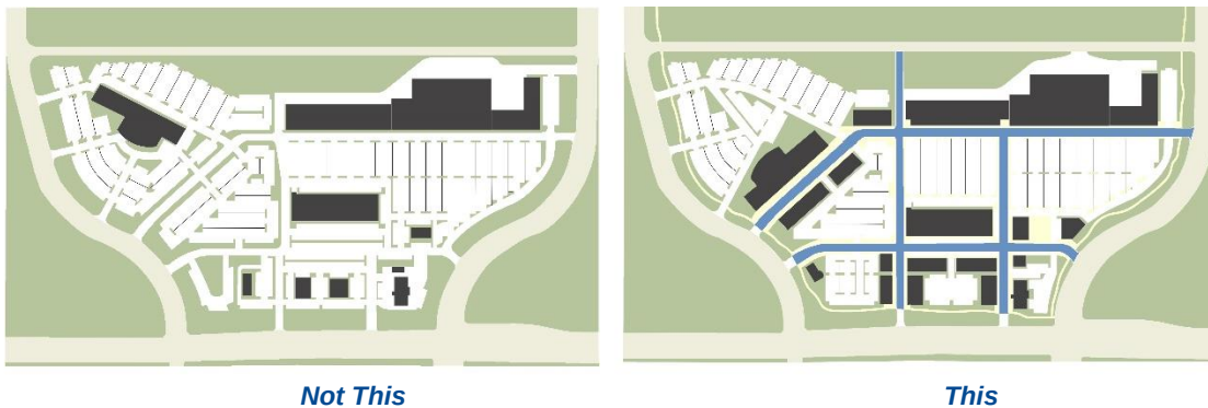
Figure 24-7-1: Internal access streets.
