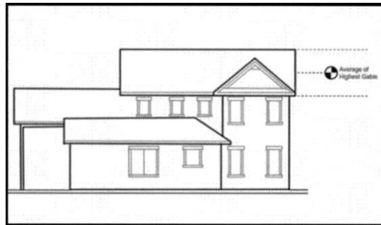
Gable Roof (2 or more gables)
