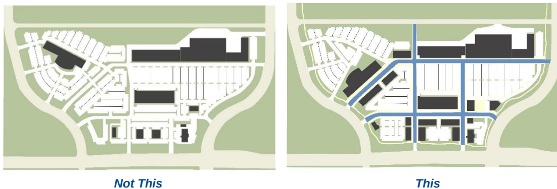
Figure 24-3-2 Internal Access Streets. Internal access streets used to mimic public street networks and streetscapes for over-sized parcels and large scale development (24-301.b.2.(d)).
